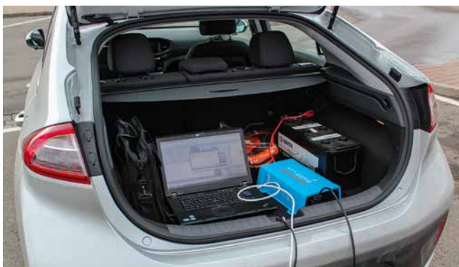
Laboratory in your case: Laptop, inverter (12V to 230V) and battery. (Components not supplied by comemso.)
