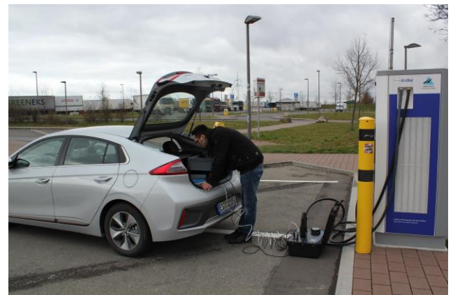
Compact and robust design for comfortable outdoor use (here: DC-CCS test).
