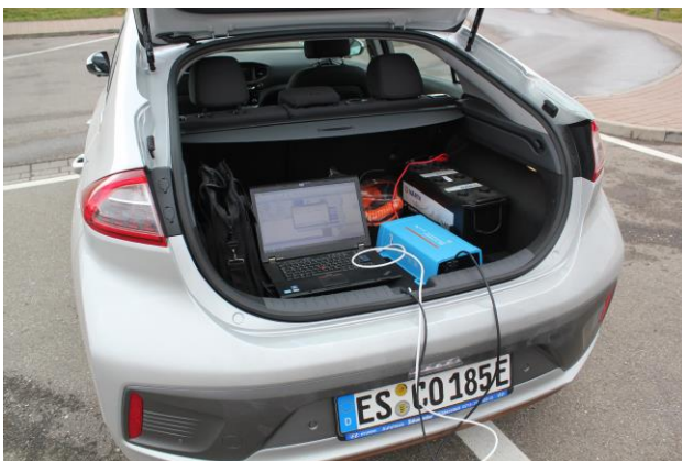
Laboratory in a trunk: Laptop, inverter (12V to 230V) and battery*.
